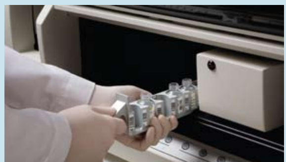
Real-time reagent management with onboard barcode reader.
