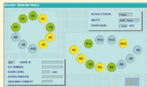
Material map provides a graphical display of reagent status.
