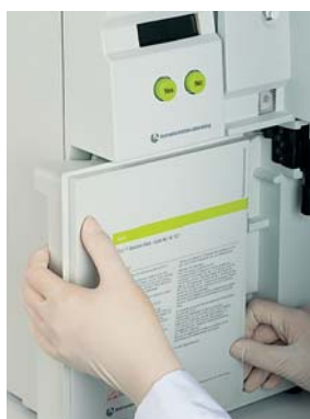
All necessary reagents and waste reservoir are contained in a one-step, plug-in disposable pack.
