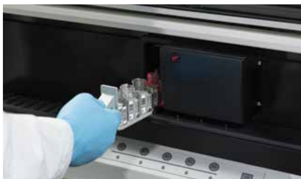
Onboard barcode reader allows real-time reagent management.
